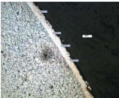
Fig. 5 — Substantially thicker white layer (0.000606 to 0.0006937 in. thick) with some developed porosity at the surface. 500x
