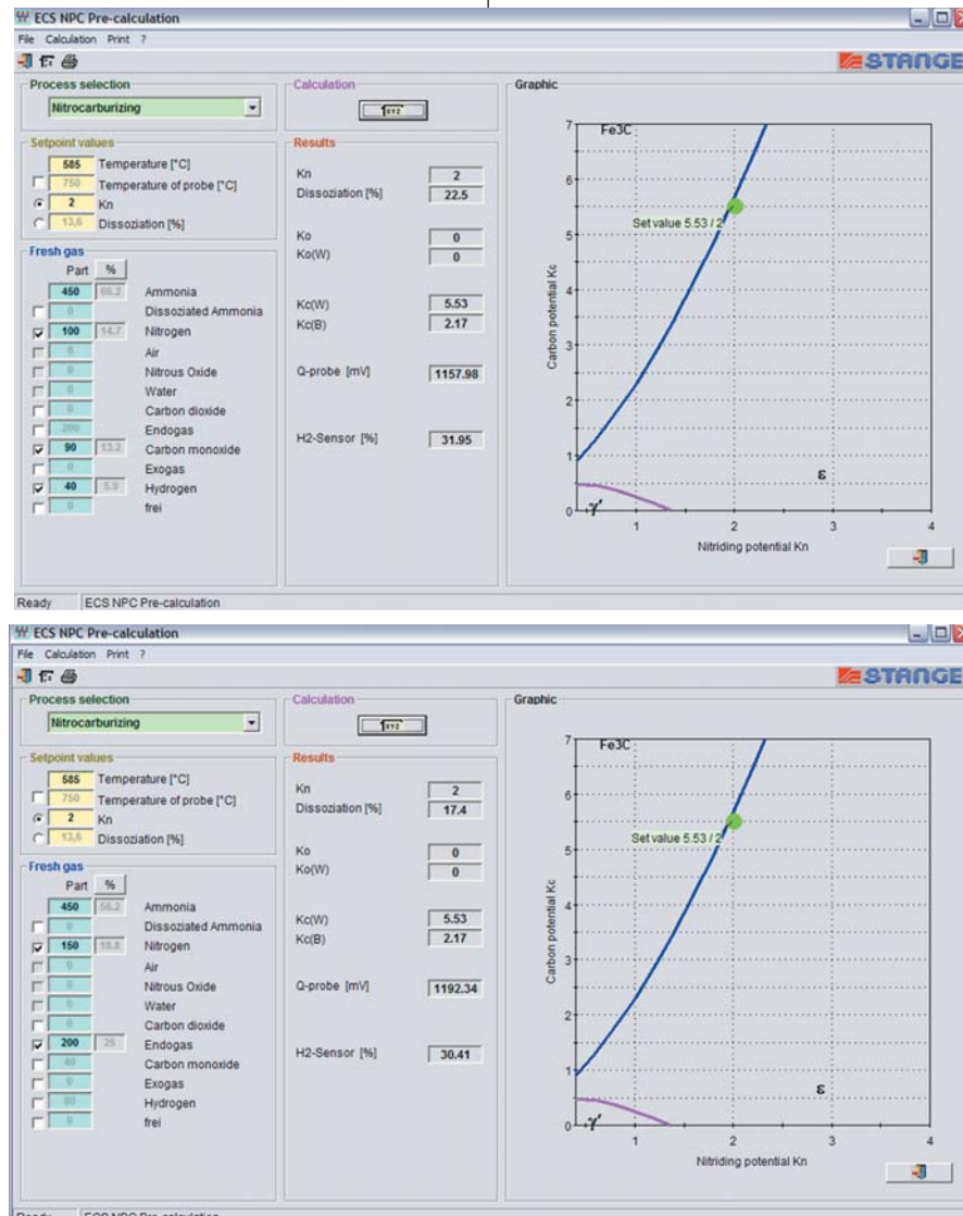
Fig. 3 — Modules for two different process gas mixtures achieving the same equilibrium relationship to the material. Charts are single-temperature representations of the tertiary Kunze diagram for nitrogen and carbon equilibrium in the steel. Inputs and outputs to the calculation tool include process gas type, flow rates, operating temperature, and nitriding potential ( K_n ).
