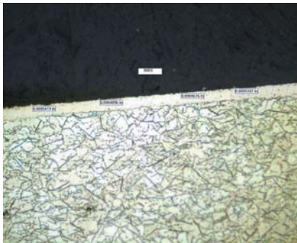
Fig. 4 — Very uniform white layer (0.0004676 to 0.0005419 in. thick) with limited porosity at the surface of the sample. 500x
