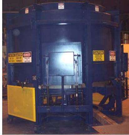
Rotary Hearth Furnace
