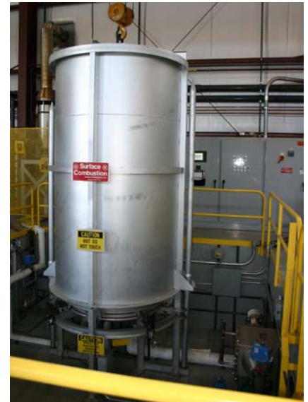
Gas Nitriding System Courtesy of Advanced Heat Treat, Monroe, MI
