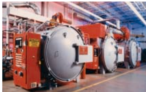
Fig 3 Lab vacuum furnaces used for carburizing testing
