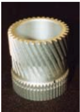
Fig 1 Typical surface quality on vacuum carburized gear
