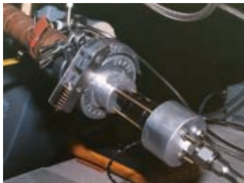
Fig 2 Liquid-hydrocarbon injector mounted to a standard K-25 inlet. Also shown are a simple two-wire 12 VDC electrical connection and a 1/4-in. stainless steel-reinforced supply hose.
