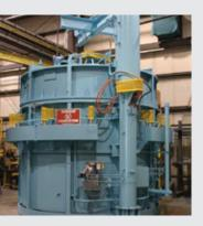
Processes performed in pit furnaces can vary from short cycle quench and temper, to deep case carburizing cycles exceeding 2-3 weeks in duration.
