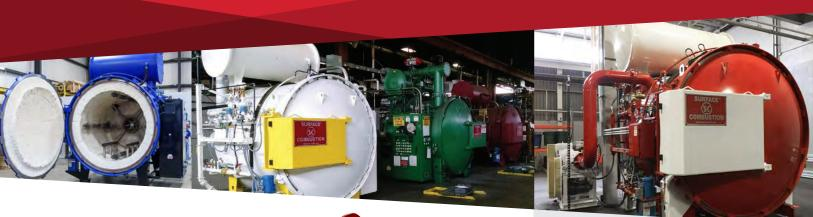
Surface Combustion is the only manufacturer in the industry to offer a low temperature vacuum purged tempering furnace. The design, featuring our patented wind flow, uniformly recirculates inert gas throughout the workload providing uniform heating and cooling.
