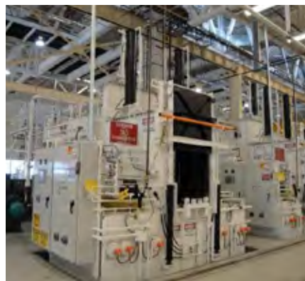
The Allcase® batch integral quench furnace was named for the ability to perform almost “all case” hardening processes.
