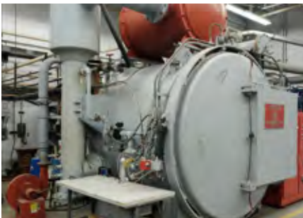
Surface Combustion single chamber vacuum carburizing furnace located in the Maumee, Ohio R&D facility.
