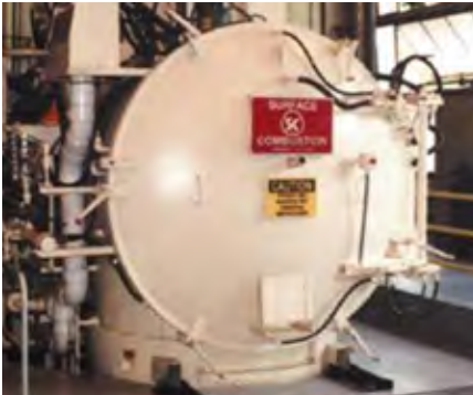
Two chamber vacuum carburizing furnace with oil quench capabilities.
