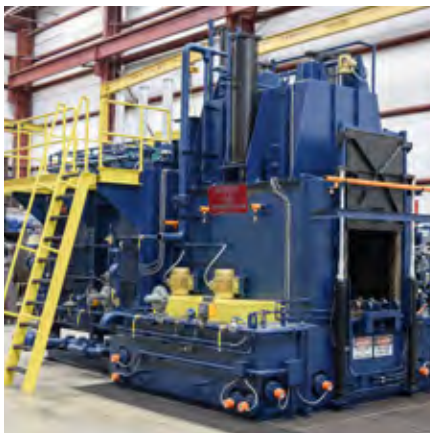
Many times, the Allcase® batch integral quench furnace design is supplied with the capability of trinitriding™ or the ferritic nitrocarburizing process.
