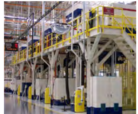
Multiple (4) vertical bottom load type ion nitriding furnaces used for high production demands.
